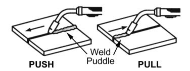
For most welding jobs you will pull the torch along the weld joint to take advantage of the greater weld puddle visibility.
