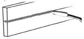
VERTICAL POSITION It is easier for many people to Pull the torch from top to bottom. It can be difficult to prevent the puddle from running downward. Pushing the torch from bottom to top may provide better puddle control and allow slower rates of travel speed to achieve deeper penetration. When vertical welding, angle B (see HOLDING THE TORCH) is usually always kept at zero, but angle A will generally range from 45 to 60 degrees to provide better puddle control.
