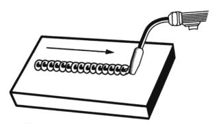
The WEAVE BEAD Used when you want to deposit metal over a wider space than would be possible with a stringer bead. It is made by weaving from side to side while moving with the torch. It is best to hesitate momentarily at each side before weaving back the other way.
