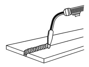
HORIZONTAL POSITION Is performed very much the same as the flat weld except that angle B (see HOLDING THE TORCH) is such that the wire, directed more toward the metal above the weld joint is to help prevent the weld puddle from running downward while still allowing slow enough travel speed. A good starting point for angle B is about 30 degrees DOWN from being perpendicular to the work piece.
