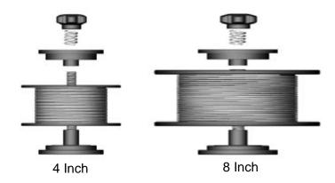
4.2.6 Setting the wire spool tension. a) Turn the spool of wire with one hand. b) Increase the spool tension by tightening (turn clockwise) the wing nut while turning the spool. Turn the spool while tightening the wing nut until the spool slows down and you feel a slight drag. Stop tightening the wing nut, you may need to repeat these steps until proper spool tension is achieved.
