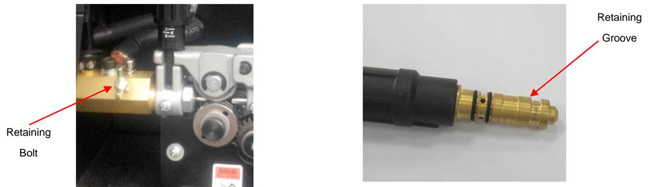
1.3 Insert the back end of the MIG torch into the MIG socket on the front of your machine. Make certain to completely slide the torch all the way in. Slightly twist to assist with pushing the torch to the back of the receptacle. The retaining bolt can then be tightened, making certain the bolt sets down into the retaining groove on the back of the MIG torch.
