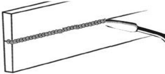
**VERTICAL POSITION** It is easier for many people to Pull the torch from top to bottom. It can be difficult to prevent the puddle from running downward. Pushing the torch from bottom to top may provide better puddle control and allow slower rates of travel speed to achieve deeper penetration. When vertical welding, angle B (see **HOLDING THE TORCH**) is usually always kept at zero, but angle A will generally range from 45 to 60 degrees to provide better puddle control.
