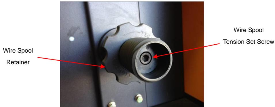
4.2.6 Setting the wire spool tension. a) Turn the spool of wire with one hand. b) Increase the spool tension by tightening (turn clockwise) the Wire Spool Tension Set Screw while turning the spool. Turn the spool while tightening the Wire Spool Tension Set Screw until the spool slows down and you feel a slight drag. Stop tightening the Wire Spool Tension Set Screw, you may need to repeat these steps until proper spool tension is achieved.
